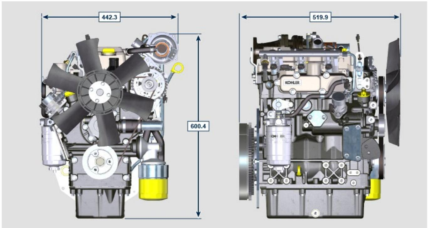
**NOTE :** Dimensions vary according to engine configuration.
