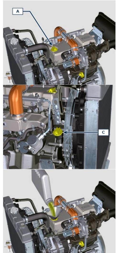
3. Before checking oil engine needs to be level.
