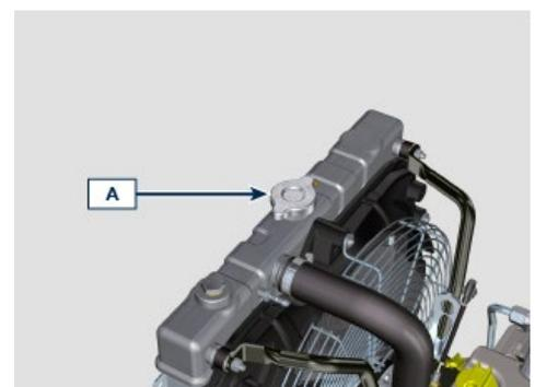
5. Keep it running at idle speed until the cooling liquid level goes down and becomes steady (the waiting times varies according to the ambient temperature).
