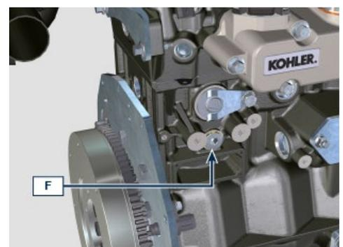
5. Tighten the drain oil plug **F** (tightening torque at **35 Nm**).
